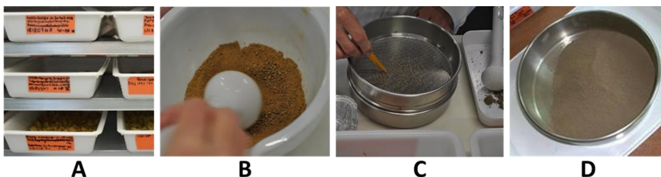
Figure 12. Sample preparation. A) drying the sample; B) crumbling clods and aggregates; C) removing coarse elements and living plant material during sieving step; D) fine earth.
