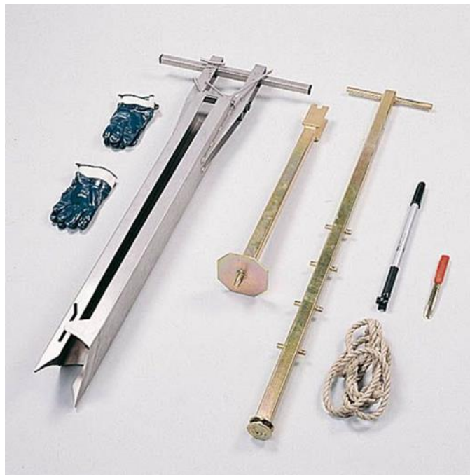
Figure 11. The Wardenaar corer designed to sample peat profiles
